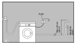
Make sure that it is designed in such a way, that the end of the drain hose cannot be covered with water.
